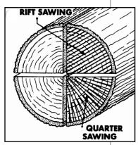
lumber, in which nearly all of the wood is verticalgrained. Also, since flat-grained wood is less dimensionally stable than vertical-grained, plainsawn lumber will tend to expand and contract more across the width of the boards than quartersawn lumber.
